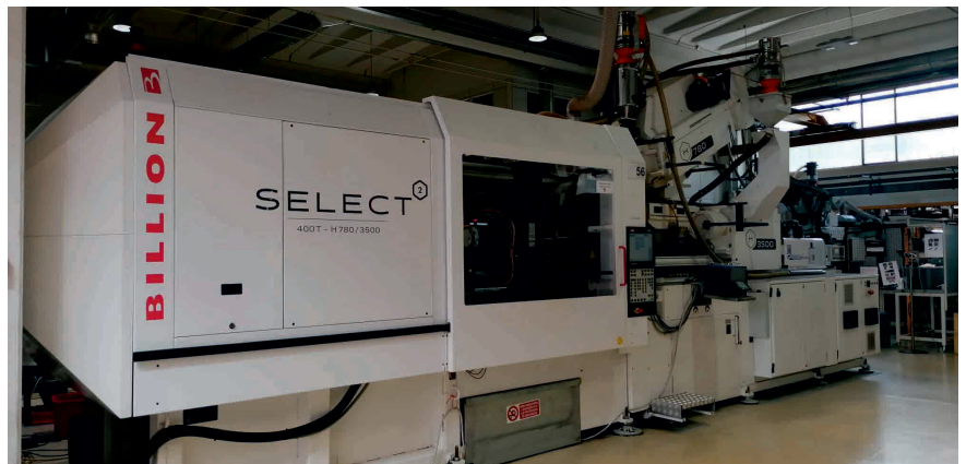
A Billion Select 2 twin-shot 400 T injection molding machine at the Techpol factory. © Billion
